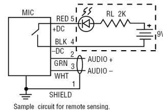
Sample circuit for remote sensing.
