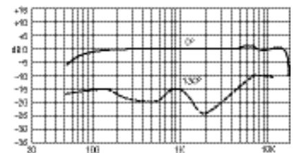
Fig. 2. Horizontal-Plane Polar Response
