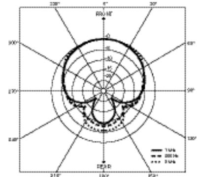
Fig. 3. Vertical-Plane Polar Response
