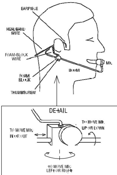
3. Now bend the headband wire to fit your head. Put the foam-block wire behind your ear. Then you can bend the earpieces to fit snugly around your ears. The back of the headband should fit firmly against the back of your neck.
